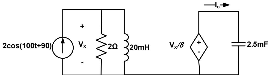
$$V_x = \frac{I_{in}}{Z_{RL}} = 2\angle 90 * \frac{4j}{2 + 2j} = 2\angle 90 * \sqrt{2}\angle -45 = 2\sqrt{2}\angle 45V$$
