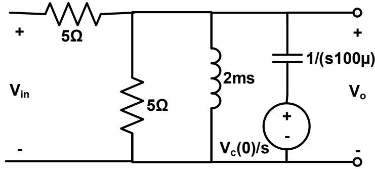
$$V_c(0^-) = \frac{5}{5+5} V_{in} = 0.5V_{in}$$
