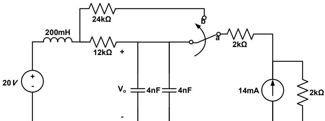
For all the time prior to zero, the switch is at position (a), at  $t=0$  the switch was moved to position (b).
